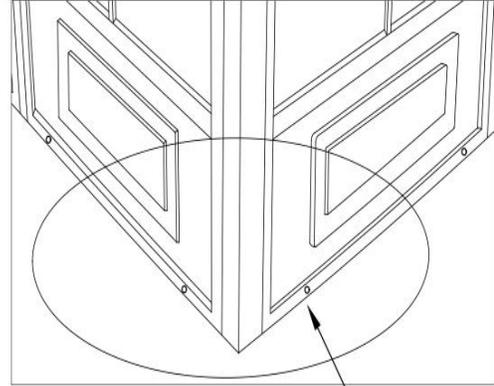
On the outside face, it is suggested to drill holes at the bottom end of the panels to permit drainage when installing on concrete floor
