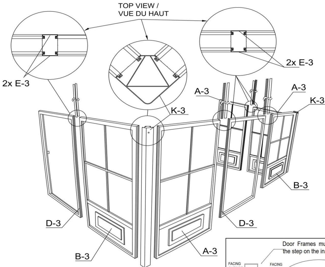
**NOTE:** When sliding the connectors, shake the frame so that they will slide easily. Do not use tools of force. If needed, clean the paint with a file and make sure the ends of the frame and joints are not bent or wrapped. If so, use the needle-nosed pliers to straighten or a file to make them slide easily.
