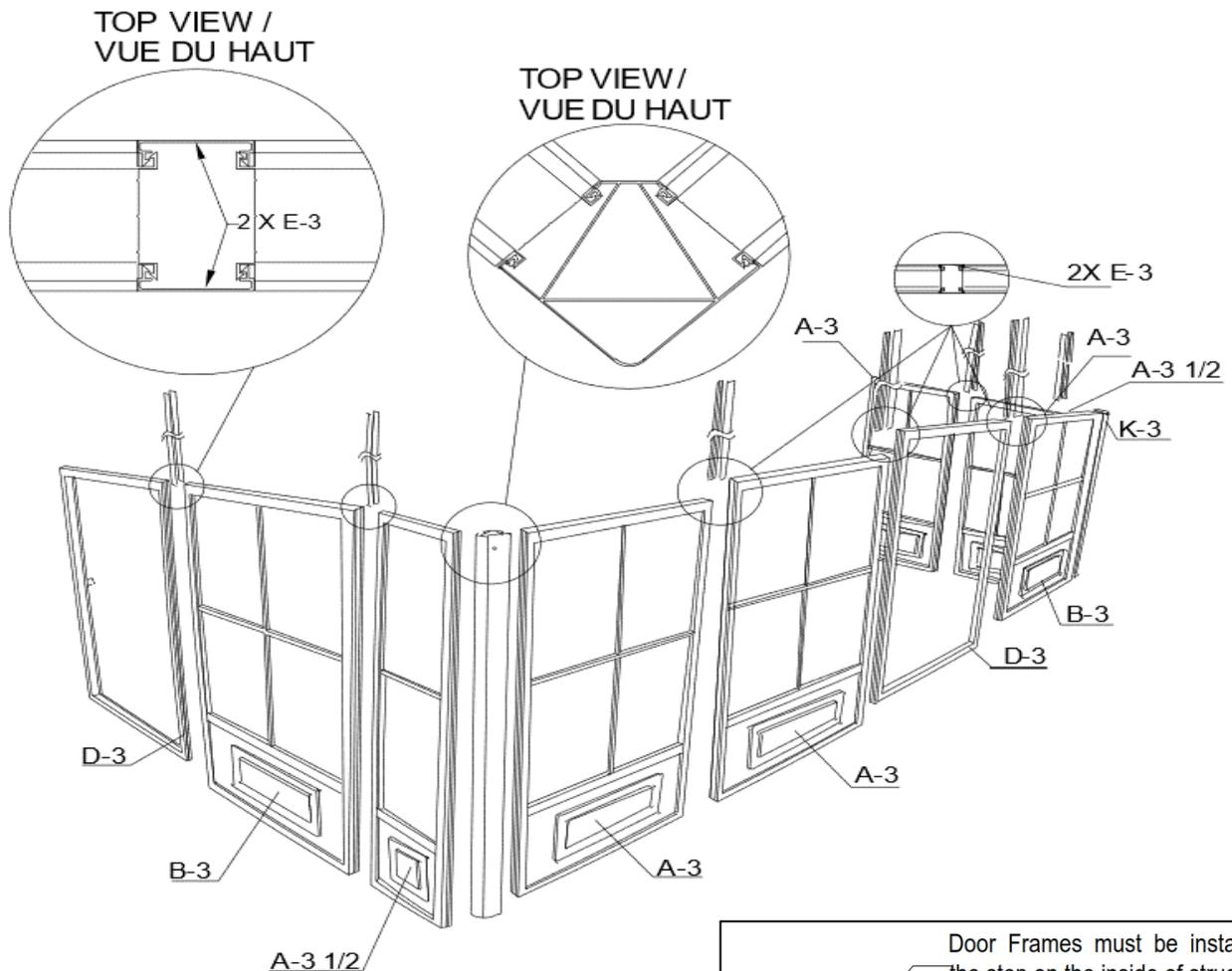
**NOTE:** When sliding the connectors, shake the frame so that they will slide easily. Do not use tools to force. If needed, clean the paint with a file and make sure the ends of the frame and joints are not bent or warped. If so, use the needle-nosed pliers to straighten.
