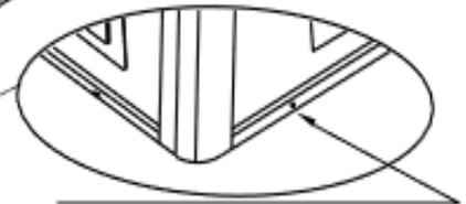
On the outside face, it is suggested to drill holes at the bottom end of the panels to permit drainage when installing on concrete floor /
